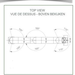
Monitor fitting: Philips Intellivue series Color: Decorative parts: RAL 5013 cobalt blue Aluminium parts: RAL 9016 traffic white Max. load capacity of support arm: 8 kg Monitor fitting max. load: 8 Kg Product weight: 2,8 Kg
