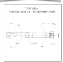
Monitor fitting: Philips Intellivue series Colour: Decorative parts: RAL 5013 cobalt blue Aluminium parts: RAL 9016 traffic white Max. load capacity of support arm: 18 kg Monitor fitting max. load: 18 Kg Product weight: 3,1 Kg
