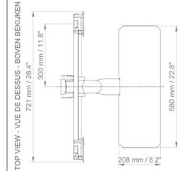
Monitor fitting: VESA 75/100 mm Color: Decorative parts: RAL 5013 cobalt blue Aluminium parts: RAL 9016 traffic white Balance scale of this medical arm: 10,5 - 18 Kg Product weight: 13 Kg Maximum weight per screen: 8 Kg Height adjustment: parallel mechanism for a constant viewing angle Safety: Has a safety stop button for height adjustment, which allows the medical arm to stay in the chosen position.
