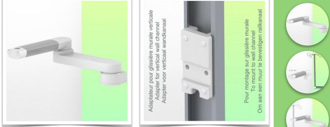
This double swivel arm for infusion pump stands is standard with a length of 554 mm and allows a 25 mm diameter infusion pole or a pole with the same diameter to be fixed, oriented and adjusted perfectly. Rotation axis from the fixing: 90° to the right and 90° to the left. Central axis between the two arms 180° rotation
