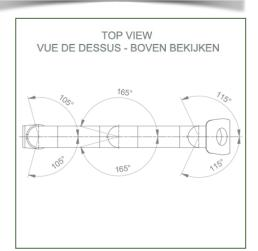
Monitor fitting: 5" Plunge plate of Quick Release Color: Decorative parts: RAL 5013 cobalt blue Aluminium parts: RAL 9016 traffic white Max. load capacity of support arm: 8 kg Monitor fitting max. load: 8 Kg Product weight: 2,8 Kg
