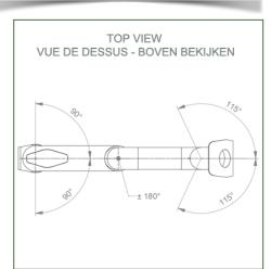
Monitor fitting: 5" Plunge plate or Quick Release Color: Decorative parts: RAL 5013 cobalt blue Aluminium parts: RAL 9016 traffic white Max. load capacity of support arm: 18 kg Monitor fitting max. load: 18 Kg Product weight: 3,1 Kg
