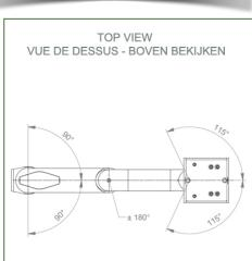
Monitor fitting: 5" Plunge plate Color: Decorative parts: RAL 5013 cobalt blue Aluminium parts: RAL 9016 traffic white Max. load capacity of support arm: 18 kg Monitor fitting max. load: 18 Kg Product weight: 3,1 Kg
