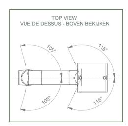
Monitor attachment: 5" immersion plate Color: Decorative parts: RAL 5013 cobalt blue Aluminium parts: RAL 9016 traffic white Max. load capacity of support arm: 18 kg Monitor attachment max. load capacity: 18 Kg
