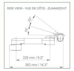
Monitor fitting: 5" Plunge plate or Quick Release Color: Decorative parts: RAL 5013 cobalt blue Aluminium parts: RAL 9016 traffic white Max. load capacity of support arm: 18 kg Monitor fitting max. load: 18 Kg Product weight: 1,9 Kg
