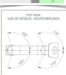
Monitor fitting: 5" Plunge plate or Quick Release Colour: Decorative parts: RAL 5013 cobalt blue Aluminium parts: RAL 9016 traffic white Max. load capacity of support arm: 18 kg Monitor fitting max. load: 18 Kg Product weight: 1,9 Kg
