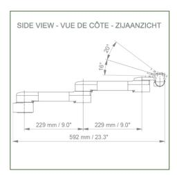
Monitor fitting: 5" Plunge plate or Quick Release Colour: Decorative parts: RAL 5013 cobalt blue Aluminium parts: RAL 9016 traffic white Max. load capacity of support arm: 18 kg
