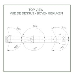
Monitor adaptation: Diving plate 5" Color: Decorative parts: RAL 5013 cobalt blue Aluminum parts: RAL 9016 traffic white Max load capacity. support arm: 8 kg Max load monitor adaptation: 8 kg Product weight: 2.8 kg
