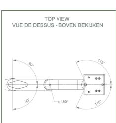
Monitor adaptation: Diving plate 5" Color: Decorative parts: RAL 5013 cobalt blue Aluminum parts: RAL 9016 traffic white Max load capacity. support arm: 18 kg Max load monitor adaptation: 18 kg Product weight: 3.1 kg
