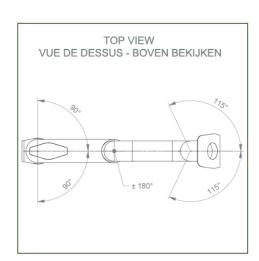
Monitor adaptation: Diving plate 5" oe Quick release Color: Decorative parts: RAL 5013 cobalt blue Aluminum parts: RAL 9016 traffic white Max load capacity. support arm: 18 kg Max load monitor adaptation: 18 kg Product weight: 3.1 kg
