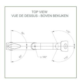
Monitor adaptation: Diving plate 5" or quick release Color: Decorative parts: RAL 5013 cobalt blue Aluminum parts: RAL 9016 traffic white Max load capacity. support arm: 18 kg Max load monitor adaptation: 18 kg Product weight: 3.1 kg
