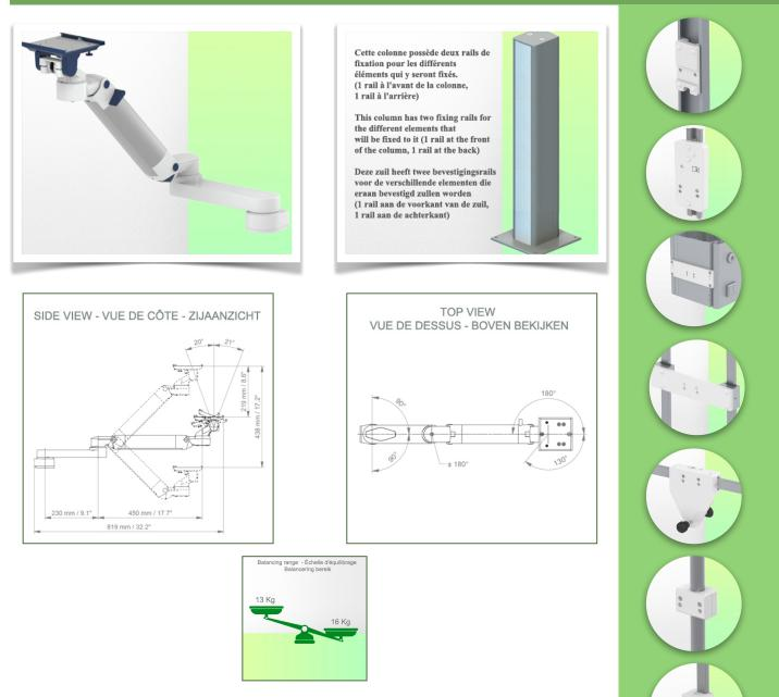
Monitor adaptation: 5" Plunge Plate Colour: Decorative parts: RAL 5013 cobalt blue Aluminium parts: RAL 9016 traffic white Max. load capacity of support arm: 22 kg Max. load monitor adaptation: 18 Kg Balancing scale for this medical arm: 13 - 16 Kg Product weight: 4,9 Kg Height adjustment: parallel mechanism for a constant viewing angle Safety: Has a safety stop button for height adjustment, allowing the medical arm to remain in the chosen position.
