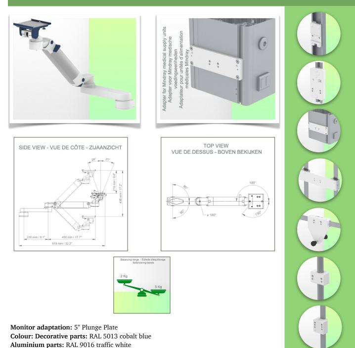
Max. load capacity of support arm: 22 kg Max. load monitor adaptation: 18 Kg
