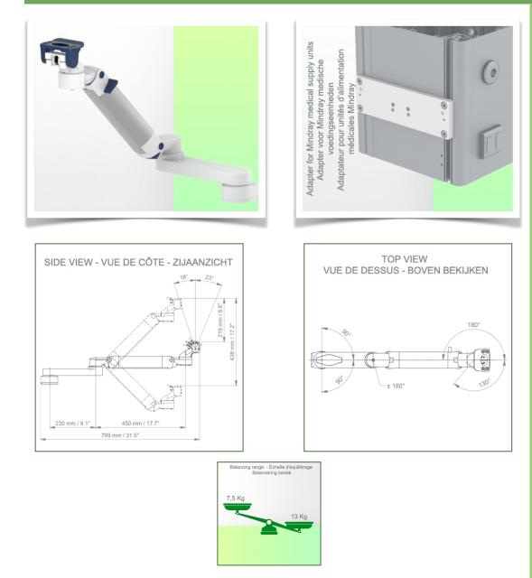
Monitor adaptation: 5" Plunge Plate or Quick Release Colour: Decorative parts: RAL 5013 cobalt blue Aluminium parts: RAL 9016 traffic white Max. load capacity of support arm: 22 kg Max. load monitor adaptation: 18 Kg Balancing scale for this medical arm: 7,5 - 13 Kg Product weight: 4,9 Kg Height adjustment: parallel mechanism for a constant viewing angle Safety: Has a safety stop button for height adjustment, allowing the medical arm to remain in the chosen position.
