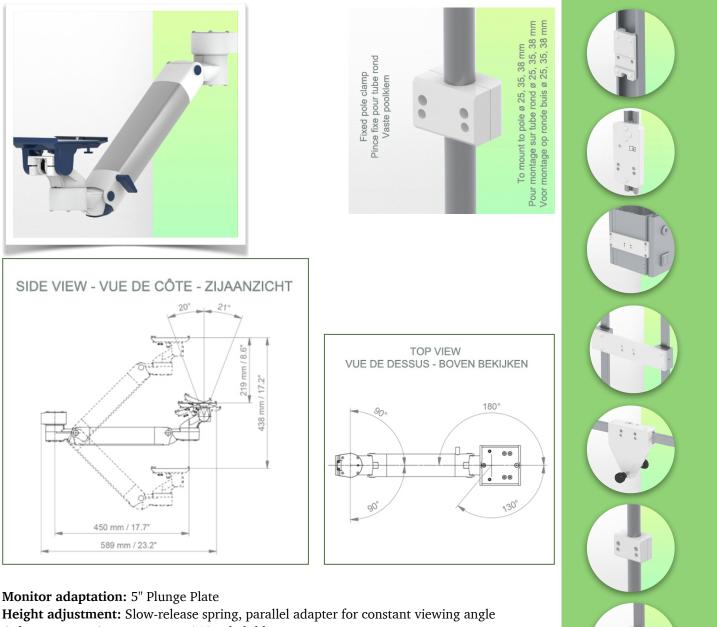
Colour: Decorative parts: RAL 5013 cobalt blue Aluminium parts: RAL 9016 traffic white Max. load capacity: 22 kg Monitor adaptation max. load: 18 Kg Balance scale on this medical arm: 4 - 9 Kg Product weight: 3.8 Kg Safety: Has a safety stop button for height adjustment, which allows the medical arm to remain in the chosen position.
