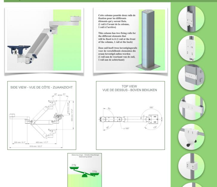
Monitor adaptation: 5" Plunge Plate Colour: Decorative parts: RAL 5013 cobalt blue Aluminium parts: RAL 9016 traffic white Max. load capacity of support arm: 22 kg Max. load monitor adaptation: 18 Kg Balancing scale for this medical arm: 2 - 5 Kg Product weight: 4,9 Kg Height adjustment: parallel mechanism for a constant viewing angle Safety: Has a safety stop button for height adjustment, allowing the medical arm to remain in the chosen position.
