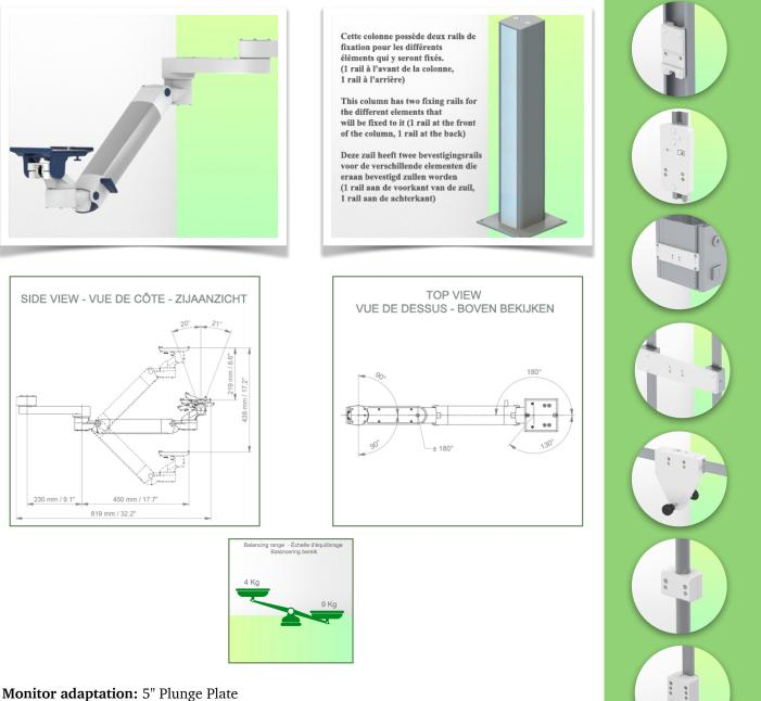
Colour: Decorative parts: RAL 5013 cobalt blue Aluminium parts: RAL 9016 traffic white Max. load capacity of support arm: 22 kg Max. load monitor adaptation: 18 Kg Balancing scale for this medical arm: 4 - 9 Kg Product weight: 4,9 Kg Height adjustment: parallel mechanism for a constant viewing angle Safety: Has a safety stop button for height adjustment, allowing the medical arm to remain in the chosen position.
