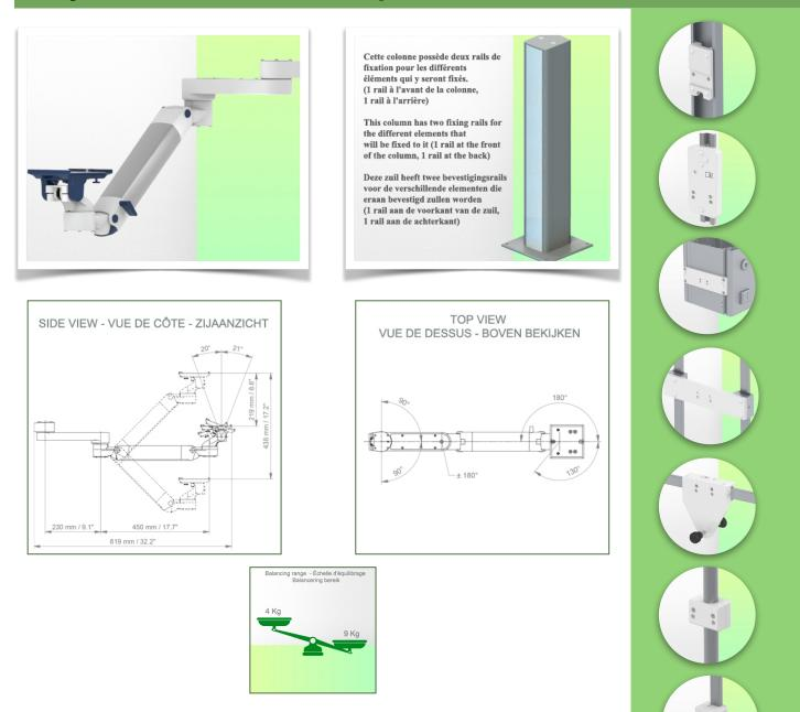
Monitor adaptation: 5" Plunge Plate Colour: Decorative parts: RAL 5013 cobalt blue Aluminium parts: RAL 9016 traffic white Max. load capacity of support arm: 22 kg Max. load monitor adaptation: 18 Kg Balancing scale for this medical arm: 4 - 9 Kg Product weight: 4,9 Kg Height adjustment: parallel mechanism for a constant viewing angle Safety: Has a safety stop button for height adjustment, allowing the medical arm to remain in the chosen position.
