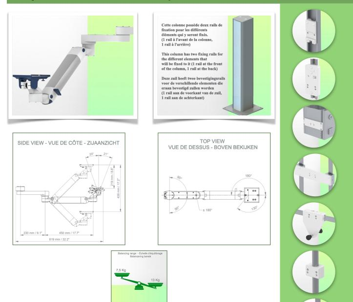
Monitor adaptation: 5" Plunge Plate Colour: Decorative parts: RAL 5013 cobalt blue Aluminium parts: RAL 9016 traffic white Max. load capacity of support arm: 22 kg Max. load monitor adaptation: 18 Kg Balancing scale for this medical arm: 7,5 - 13 Kg Product weight: 4,9 Kg Height adjustment: parallel mechanism for a constant viewing angle Safety: Has a safety stop button for height adjustment, allowing the medical arm to remain in the chosen position.
