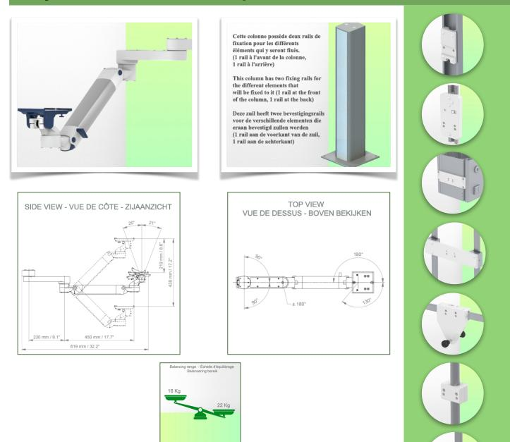
Monitor adaptation: 5" Plunge Plate Colour: Decorative parts: RAL 5013 cobalt blue Aluminium parts: RAL 9016 traffic white Max. load capacity of support arm: 22 kg Max. load monitor adaptation: 18 Kg Balancing scale for this medical arm: 16 - 22 Kg Product weight: 4,9 Kg Height adjustment: parallel mechanism for a constant viewing angle Safety: Has a safety stop button for height adjustment, allowing the medical arm to remain in the chosen position.
