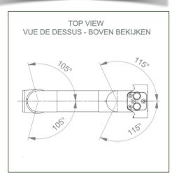
Monitor fitting: Philips Intellivue Series Color: Decorative parts: RAL 5013 cobalt blue Aluminium parts: RAL 9016 traffic white Max. load capacity of support arm: 18 kg Monitor fitting max. load: 18 Kg Product weight: 1,9 Kg
