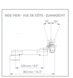
Monitor attachment: Philips Intellivue Series Color: Decorative parts: RAL 5013 cobalt blue Aluminium parts: RAL 9016 traffic white Max. load capacity of support arm: 18 kg Monitor attachment max. load capacity: 18 Kg Product weight: 1.9 Kg
