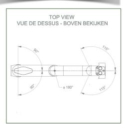
Monitor fitting: 5" Plunge plate Color: Decorative parts: RAL 5013 cobalt blue Aluminium parts: RAL 9016 traffic white Max. load capacity of support arm: 18 kg Monitor fitting max. load: 18 Kg Product weight: 3,1 Kg
