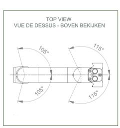
Monitor fitting: Philips Intellivue series Colour: Decorative parts: RAL 5013 cobalt blue Aluminium parts: RAL 9016 traffic white Max. load capacity of support arm: 18 kg Monitor fitting max. load: 18 Kg Product weight: 1,9 Kg
