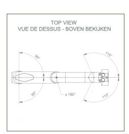
Monitor fitting: Philips Intellivue series Colour: Decorative parts: RAL 5013 cobalt blue Aluminium parts: RAL 9016 traffic white Max. load capacity of support arm: 18 kg Monitor fitting max. load: 18 Kg Product weight: 3,1 Kg
