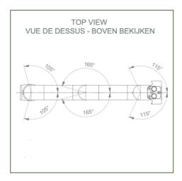
Monitor adaptation: Philips Intellivue series Color: Decorative parts: RAL 5013 cobalt blue Aluminum parts: RAL 9016 traffic white Max load capacity. support arm: 8 kg Max load monitor adaptation: 8 kg
