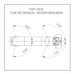
Monitor fitting: Philips Intellivue series Colour: Decorative parts: RAL 5013 cobalt blue Aluminium parts: RAL 9016 traffic white Max. load capacity of support arm: 18 kg
