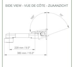
Arm fitting: Philips FMS Colour: Decorative parts: RAL 5013 cobalt blue Aluminium parts: RAL 9016 traffic white Max. load capacity of support arm: 18 kg Arm fitting max. load: 18 Kg Product weight: 1,7 Kg
