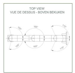
Arm fitting: Philips FMS Colour: Decorative parts: RAL 5013 cobalt blue Aluminium parts: RAL 9016 traffic white Max. load capacity of support arm: 18 kg Arm fitting max. load: 18 Kg Product weight: 2,6 Kg
