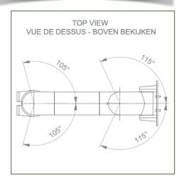
Monitor fitting: Philips Intellivue MP2/X2/X3 Series Color: Decorative parts: RAL 5013 cobalt blue Aluminium parts: RAL 9016 traffic white
