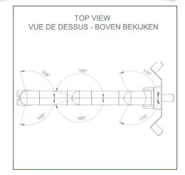
Monitor fitting: Philips Intellivue MP2/X2/X3 Series Color: Decorative parts: RAL 5013 cobalt blue Aluminium parts: RAL 9016 traffic white Max. load capacity of support arm: 8 kg Monitor fitting max. load: 8 Kg Product weight: 2,6 Kg
