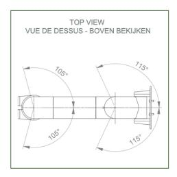
Monitor fitting: Philips Intellivue MP2/X2/X3 Series Color: Decorative parts: RAL 5013 cobalt blue Aluminium parts: RAL 9016 traffic white Max. load capacity of support arm: 18 kg
