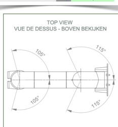
Monitor fitting: Philips Intellivue MP2/X2/X3 Series Colour: Decorative parts: RAL 5013 cobalt blue Aluminium parts: RAL 9016 traffic white Max. load capacity of support arm: 18 kg Monitor fitting max. load: 18 Kg Product weight: 1,7 Kg
