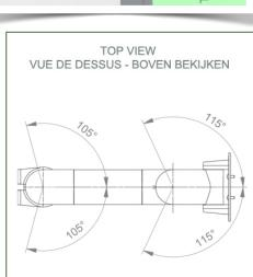
Monitor fitting: Philips Intellivue MP2/X2/X3 Series Colour: Decorative parts: RAL 5013 cobalt blue Aluminium parts: RAL 9016 traffic white Max. load capacity of support arm: 18 kg Monitor fitting max. load: 18 Kg Product weight: 2,2 Kg
