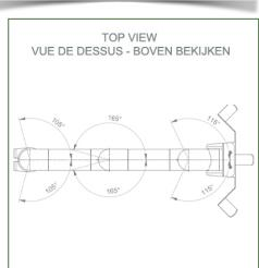
Monitor fitting: Philips Intellivue MP2/X2/X3 Series Colour: Decorative parts: RAL 5013 cobalt blue Aluminium parts: RAL 9016 traffic white Max. load capacity of support arm: 8 kg Monitor fitting max. load: 8 Kg Product weight: 3,2 Kg
