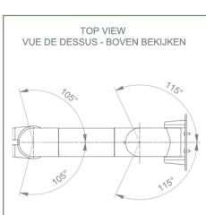
Monitor fitting: Philips Intellivue MP2/X2/X3 series Colour: Decorative parts: RAL 5013 cobalt blue Aluminium parts: RAL 9016 traffic white Max. load capacity of support arm: 18 kg Monitor fitting max. load: 18 Kg Product weight: 2,2 Kg
