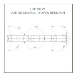
Monitor fitting: Philips Intellivue MP2/X2/X3 Series Colour: Decorative parts: RAL 5013 cobalt blue Aluminium parts: RAL 9016 traffic white Max. load capacity of support arm: 8 kg Monitor fitting max. load: 8 Kg Product weight: 2,6 Kg
