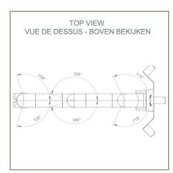
Monitor fitting: Philips Intellivue Series Colour: Decorative parts: RAL 5013 cobalt blue Aluminium parts: RAL 9016 traffic white Max. load capacity of support arm: 8 kg Monitor fitting max. load: 8 Kg Product weight: 3,2 Kg
