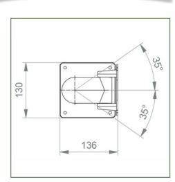
Monitor fitting: VESA 75/100 mm Colour: Decorative parts: RAL 5013 cobalt blue Screen compatibility: Up to 26" depending on the exact size of your screen and the available space on the stand height Aluminium parts: RAL 9016 traffic white Max. load capacity of the support arm: 18 kg Product weight: 1 Kg
