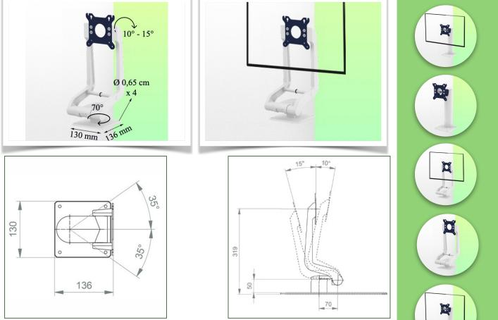
Monitor fitting: VESA 75/100 mm Colour: Decorative parts: RAL 5013 cobalt blue Screen compatibility: Up to 26" depending on the exact size of your screen and the available space on the stand height Aluminium parts: RAL 9016 traffic white Max. load capacity of the support arm: 18 kg Product weight: 1 Kg
